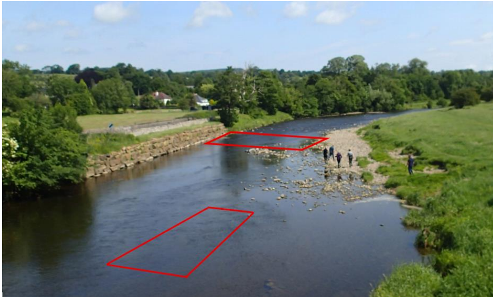
Fig. 2. The River Ribble at Bradford Bridge, showing two possible survey options for a medium or large river. The rectangle at the back shows a narrow transect; the rectangle in the foreground shows a fixed quadrat.
